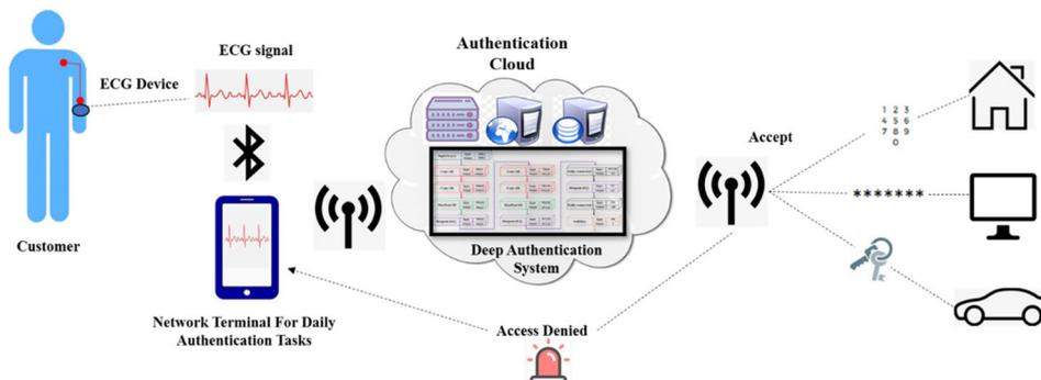
FIGURE 12 Illustration of deep authentication system using IoT. IoT, internet of things
