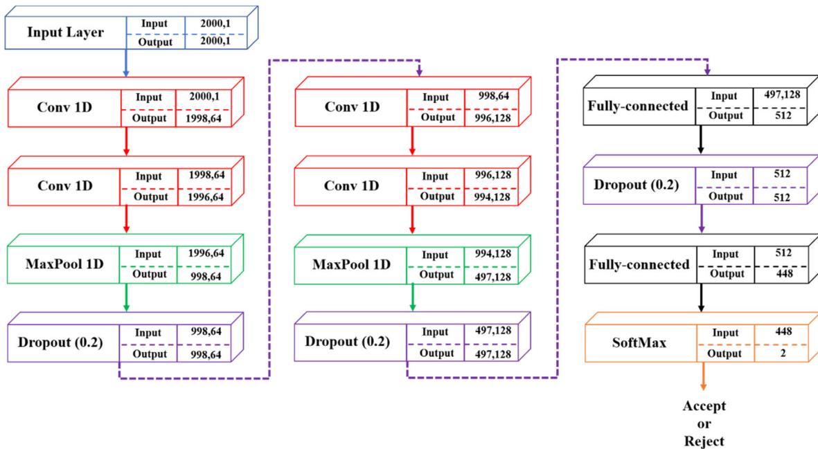
**FIGURE 5** The proposed CNN model. CNN, convolutional neural network
