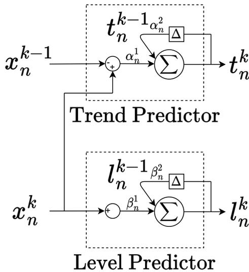
FIGURE 2: Trend and Level Predictor units of the rTPNN layer for a sensor  $n$
