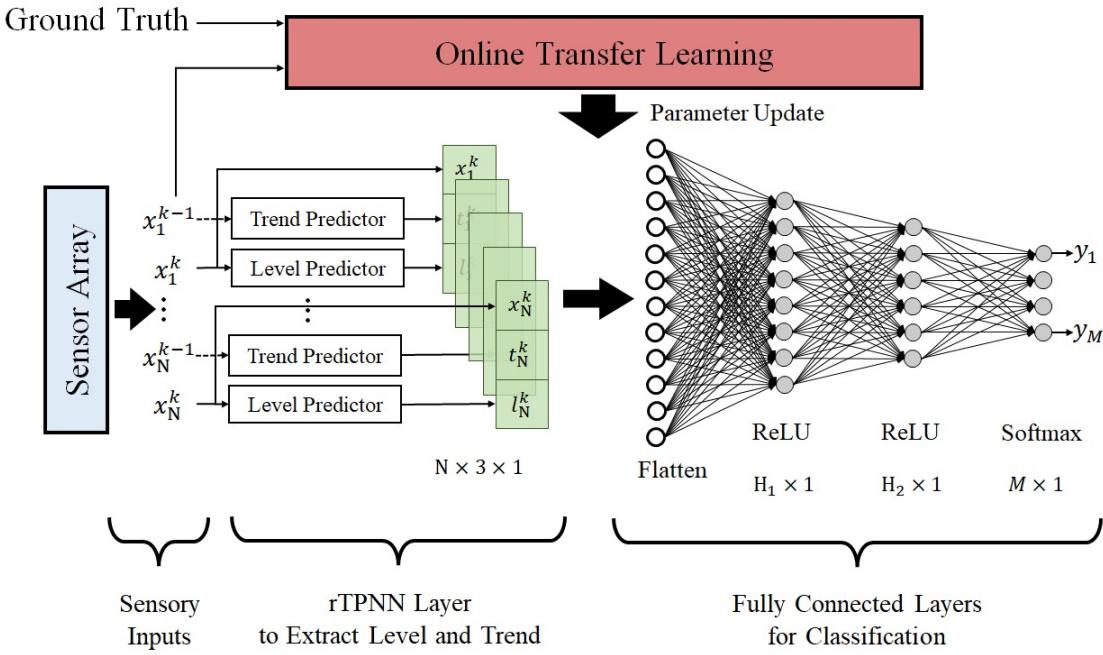
**FIGURE 1:** The architectural design of the proposed e-rTPNN decision system, which is based on the rTPNN model with online transfer learning
