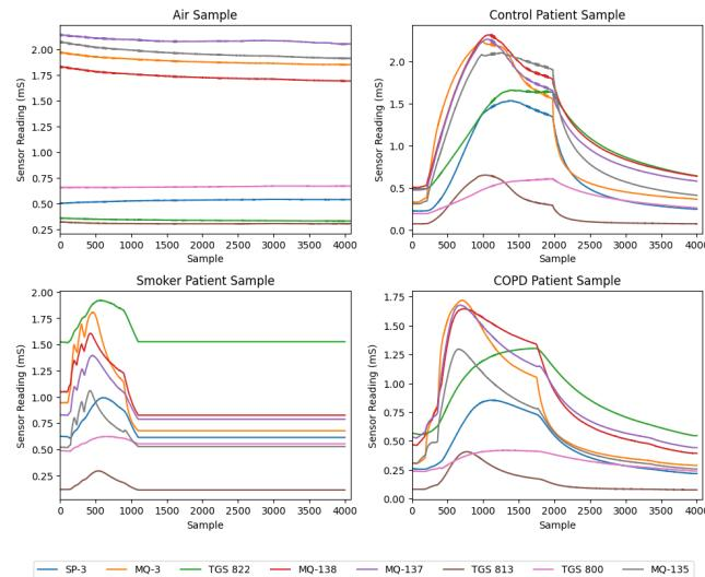
**FIGURE 4:** Exhaled breath samples acquired with the E-Nose device for AIR, COPD, Smoker and Control (healthy)
