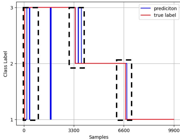
**FIGURE 5:** Model predictions vs true labels during online learning for three samples. Marked areas show wrong predictions at the start of new samples and the quick recovery of the algorithm.
