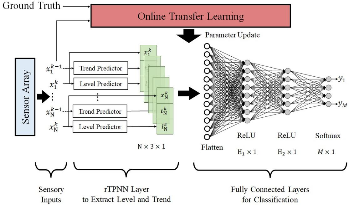
FIGURE 1: The architectural design of the proposed e-rTPNN decision system, which is based on the rTPNN model with online transfer learning
