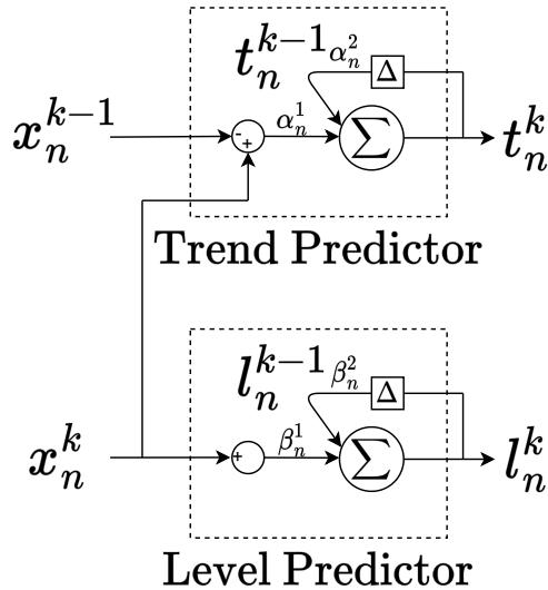
**FIGURE 2:** Trend and Level Predictor units of the rTPNN layer for a sensor  $n$
