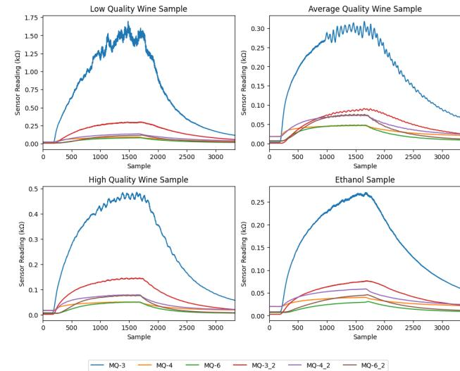
FIGURE 3: Sensor outputs for a sample wine bottles of each class.
